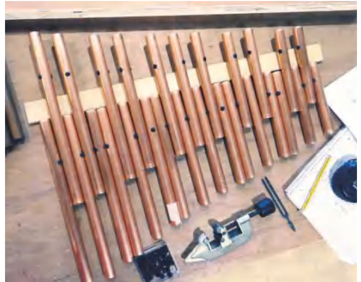
PIC 2. Tubes cut, drilled and fitted with grommets. It then occurred to me that for playability, the 'black notes' had to be positioned within reach of the 'white notes' just as they are on a piano. This gave rise to a sloping top rack. I had initially thought of making the set floor standing but that would have been a large construction and unwieldy if it were to be moved around. Rather, I made my bracket to screw to the wall
